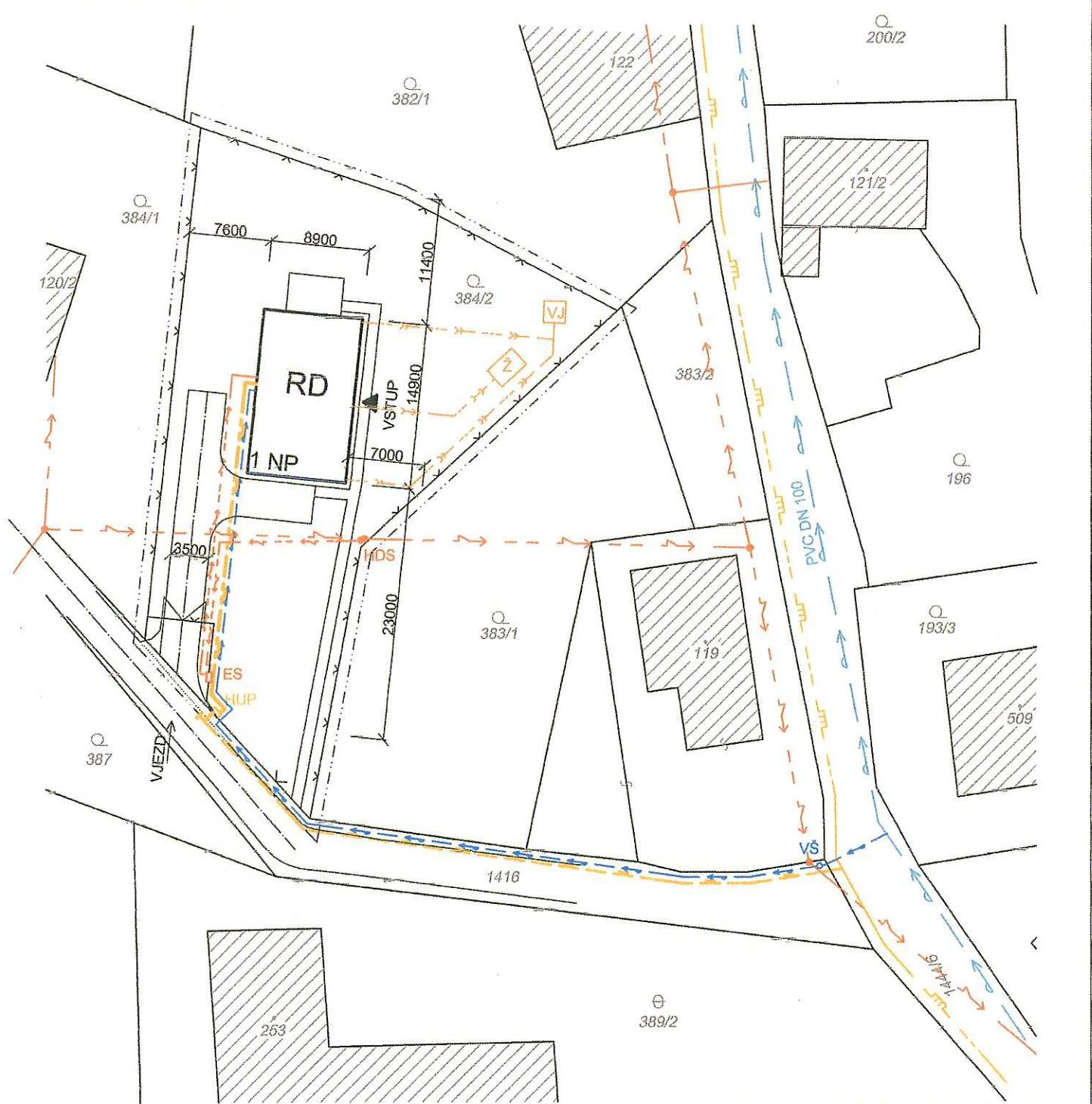
VODOVODNÍ PŘÍPOJKA HDPE D 40x3.7 MM; DL. 97.0 M
